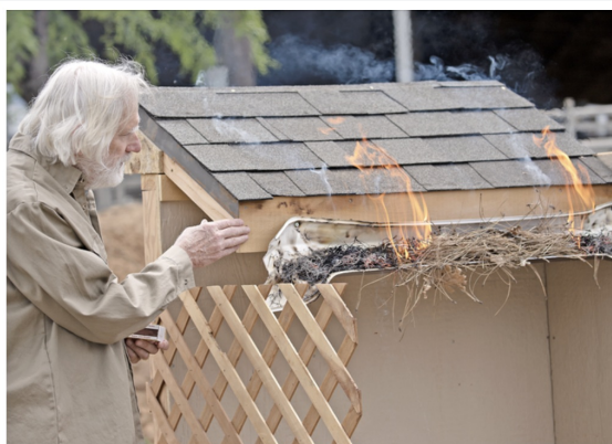
Steve Quarles demonstrates how embers can ignite dry leaf debris and melt plastic gutters. Photo by Evett Kilmartin
